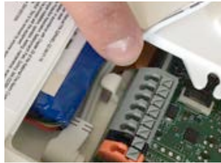
Route the wire behind the retainer clip
