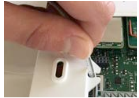
Insert the wire into the strain-relief
