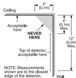
NOTE: Measurements shown are to the closest edge of the detector.
